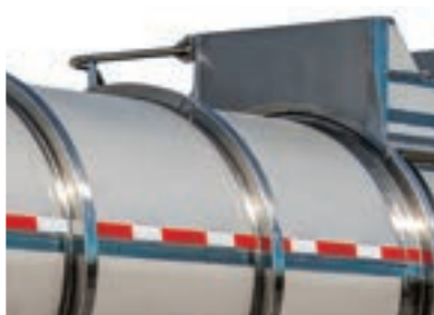
Insulated, Exposed Rings
