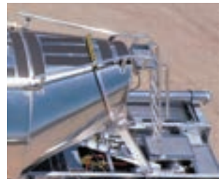
Rear Ladder with Optional Double Handrail
